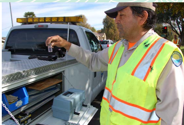
Water Systems Operator Ray Robles checks a water sample for residual disinfectant, which prevents microbial growth in the water distribution system.
