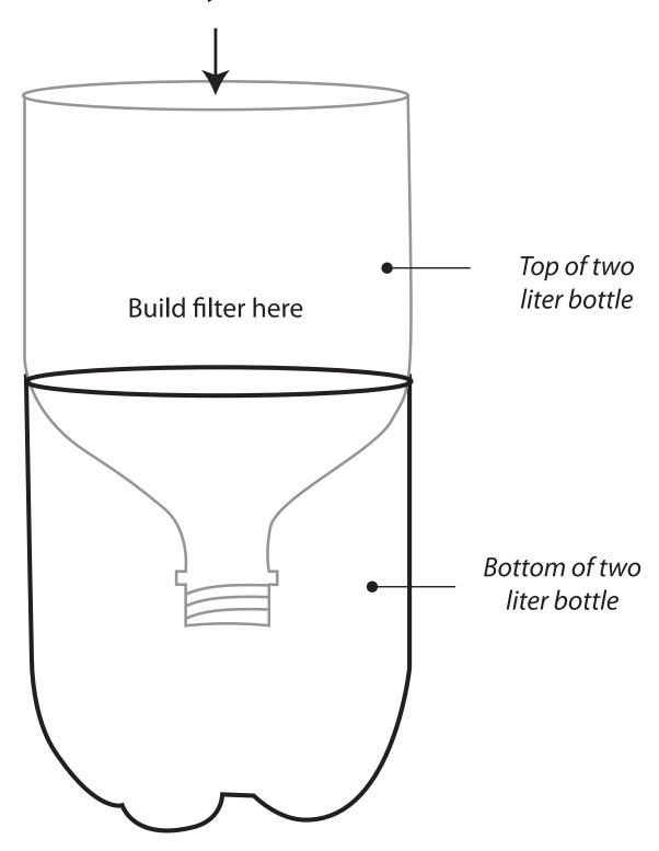
Filtered water drains into bottom of bottle
