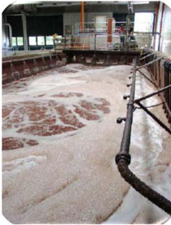
Pictures of a Deammonification Reactor (Left) and Anammox Granules from a Deammonification Reactor (Right)
