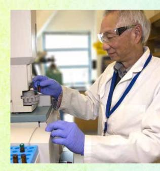
Environmental Chemist II Troy To uses a gas chromatography/mass spectrometry instrument to analyze organics to below parts per billion.
