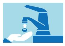
Replace all point-of-use filters, including the filter in refrigerators. Clean and reinstall or replace aerator screens.
