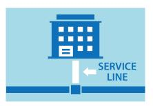
Organize flushing to maximize the flow of water (e.g., opening all outlets simultaneously to flush the service line and then flushing outlets individually starting near where the water enters the structure).
