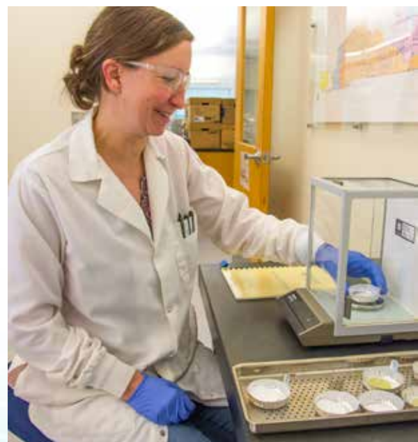
Environmental Chemist II Heidi Birdsell uses an analytical balance to weigh filters for a total suspended solids analysis.
