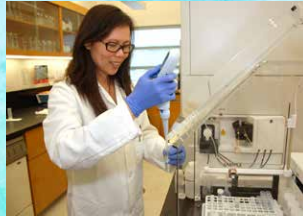
Senior Environmental Chemist Connie Sanchez prepares to load a sample for metals analysis to the Inductively Coupled Plasma-Mass Spectrometer, an instrument that detects metals such as copper and lead at the part-per-billion level.
