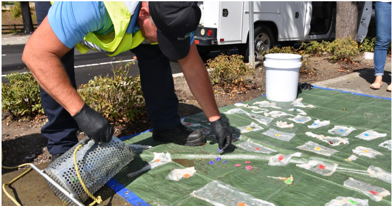
DSRSD Field Operations staff take part in a Flushable Wipes Dispersibility Field Test with the California Association of Sanitation Agencies.
